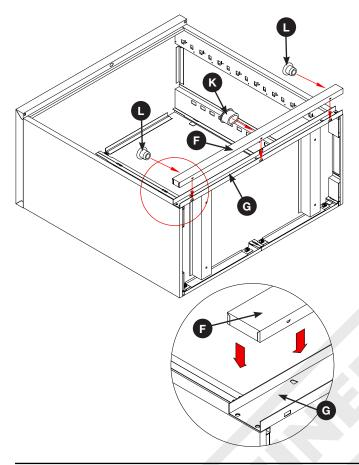
**Step 7:** Stand Cabinet upright and use 8 x Screws (M) to fix the frame together.
