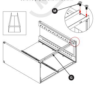
**Step 4:** Insert the base (E), then use screws (M) to secure in place as shown below.
