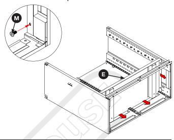
Step 5: Attach the top (D), then insert 2 x hinge plugs (L) & 1 x door lock plug (M) as shown below.
