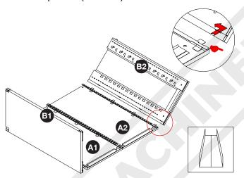
**Step 3:** Connect the inside face plate (G) with screws (M) as shown below.
